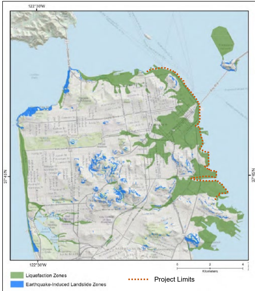
Figure B-35: California Geological Survey's Seismic Hazard Zones Map Showing Zones of Liquefaction and Earthquake-Induced Landslides
