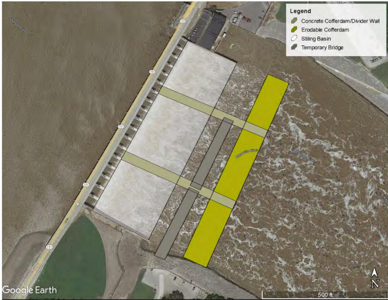
Figure 4. Bridge and Cofferdam Locations
