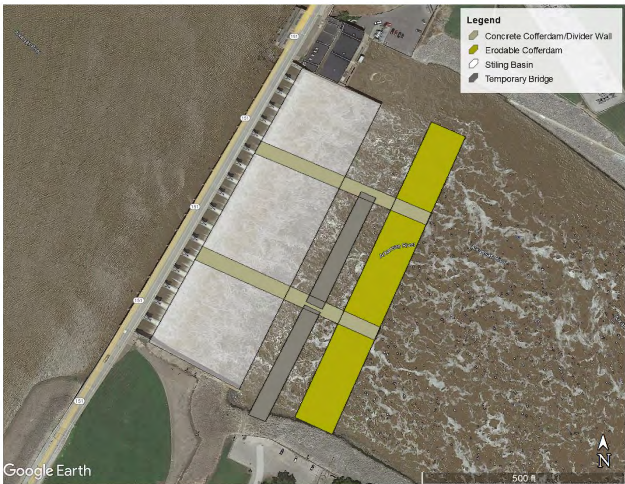
Figure 5. Bridge and Cofferdam Locations
