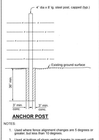
Used at bottom of sharp vertical breaks to prevent uplift from removing normally set post. EXHIBIT B
