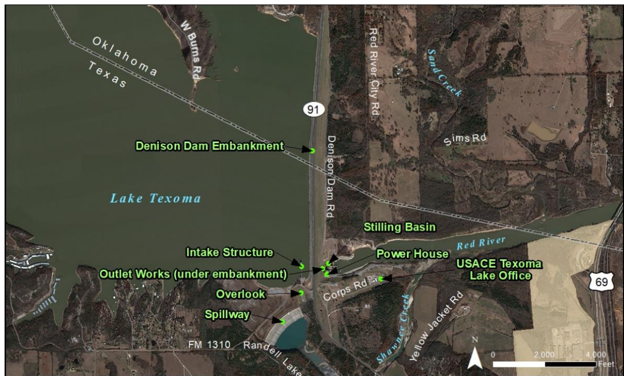
Figure 7. Overview of the Denison Dam and its components.
