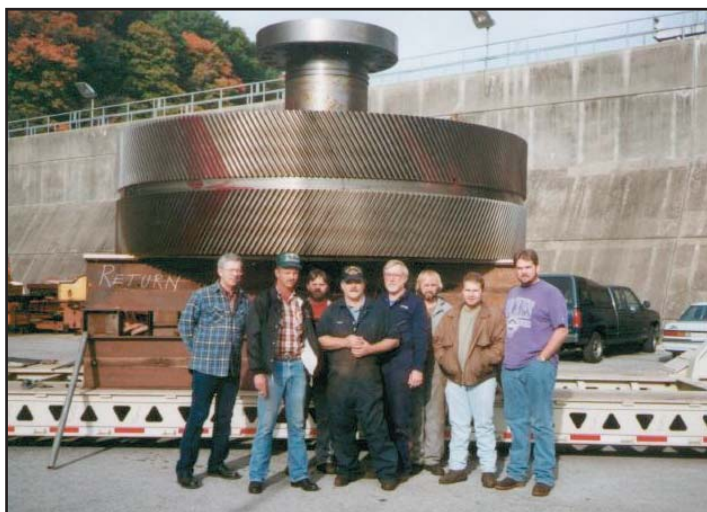
Photo of the "bullgear" taken during maintenance of the Webbers Falls powerplant in 1990.
