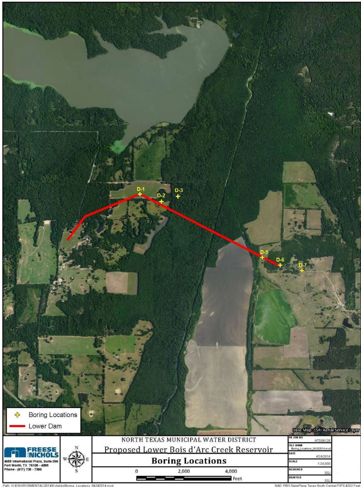
Figure 3.2-2. Location of Geotechnical Borings at Proposed LBCR Dam Site
