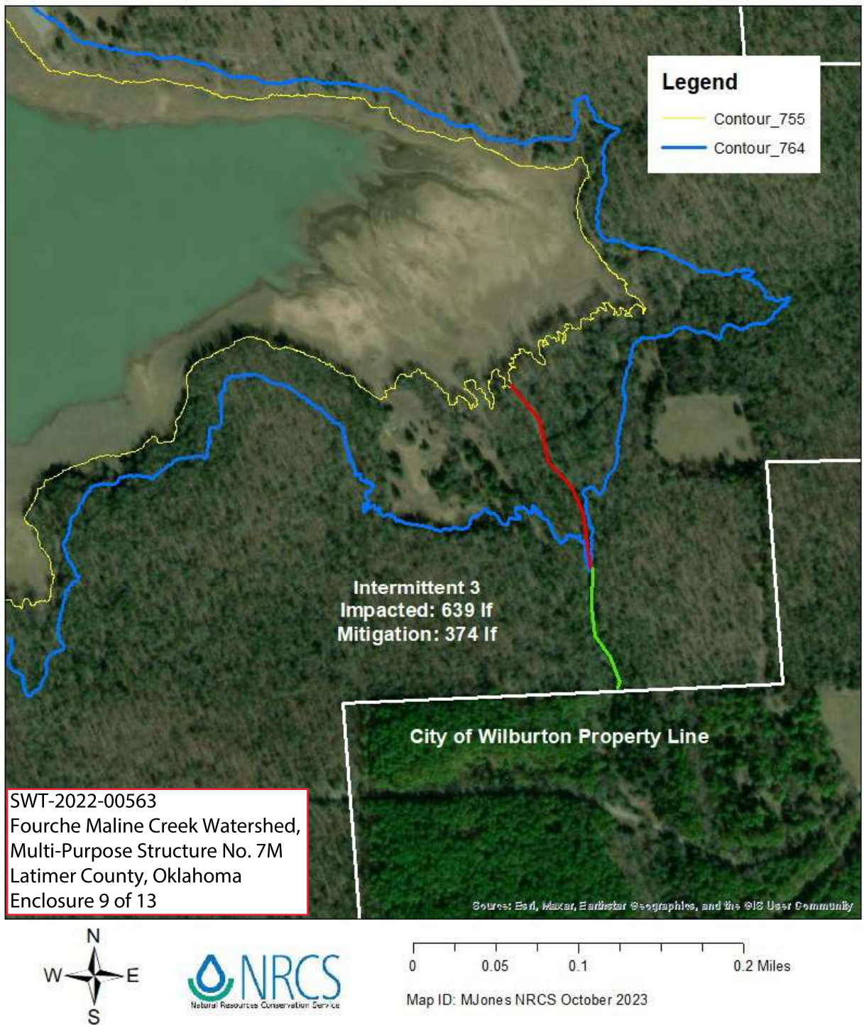
Figure 4: Intermittent stream 3. Impacted stream length was measured from existing pool elevation (contour 755) to proposed elevation (contour 764). Red is the impacted segment of stream and green is the mitigation segment of stream.
